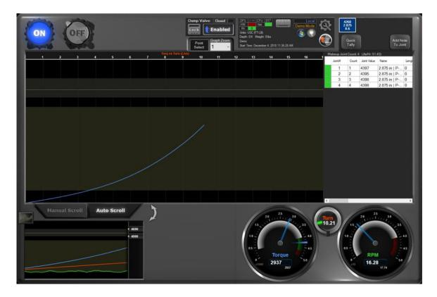
Diagram 3.4 The large graph area is Torque vs. Turns. Torque vs. Time vs. Turns vs.
