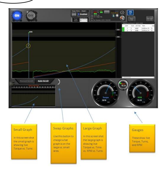
Once a job has been setup and the hardware checks are finished, Diagram 3.3 will be
