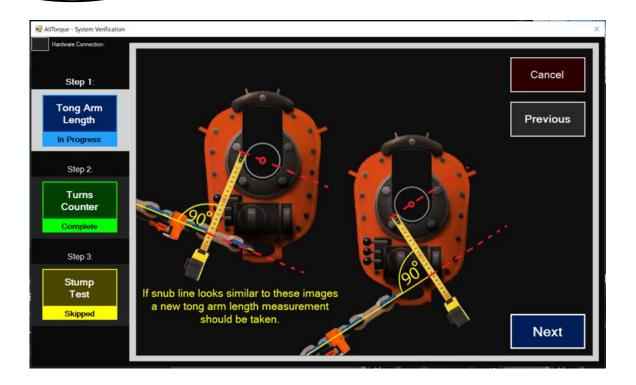
• If the snub line is connected on an angle that is +/- 15 degrees from a 90 degree angle a new tong arm length should be used. (Diagram 2.8). Excessive angles are sometimes used due to the setup of the tong on the rig floor. The excessive angles need to be compensated for as the Load Cell will notice an increased load in both cases (Diagram 2.8) The arm length can only get shorter that the 90-degree (normal) arm length.
