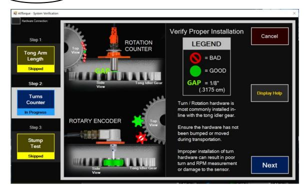
Installing a Proximity Sensor and a Rotary Turns Encoder, (Diagram 2.9).
